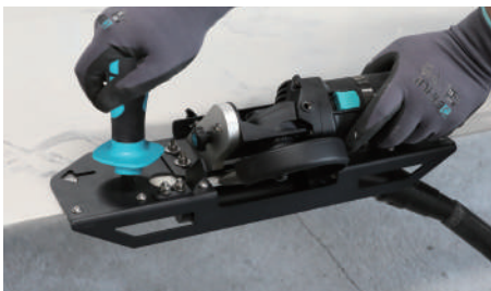
Step 3. Move forward steadily to make a perfect bevelling.
