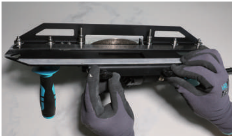
Step 2. Turn the adjusting screws in colockwise/ counterclockwise,keep both screws adjusted. Colorwise turn to get thinner cutting edge Counterclockwise to get a thicker cutting edge
