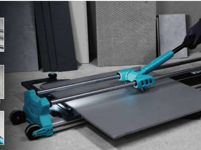
3.Snap-in for locking the handle 4.Adjustable measurement guide and side ruler
